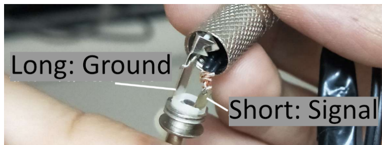
Figure 2-9 Wiring
