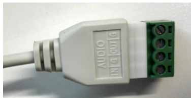
Figure 2-1 Terminal Block Audio Interface
