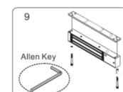
Strike the pin into the armature plate slightly (to avoid movement).
